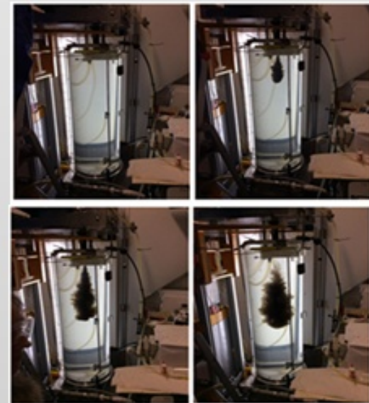
Figure 2. CEDRE Subsea Dispersant Effectiveness Test Tank in Operation
