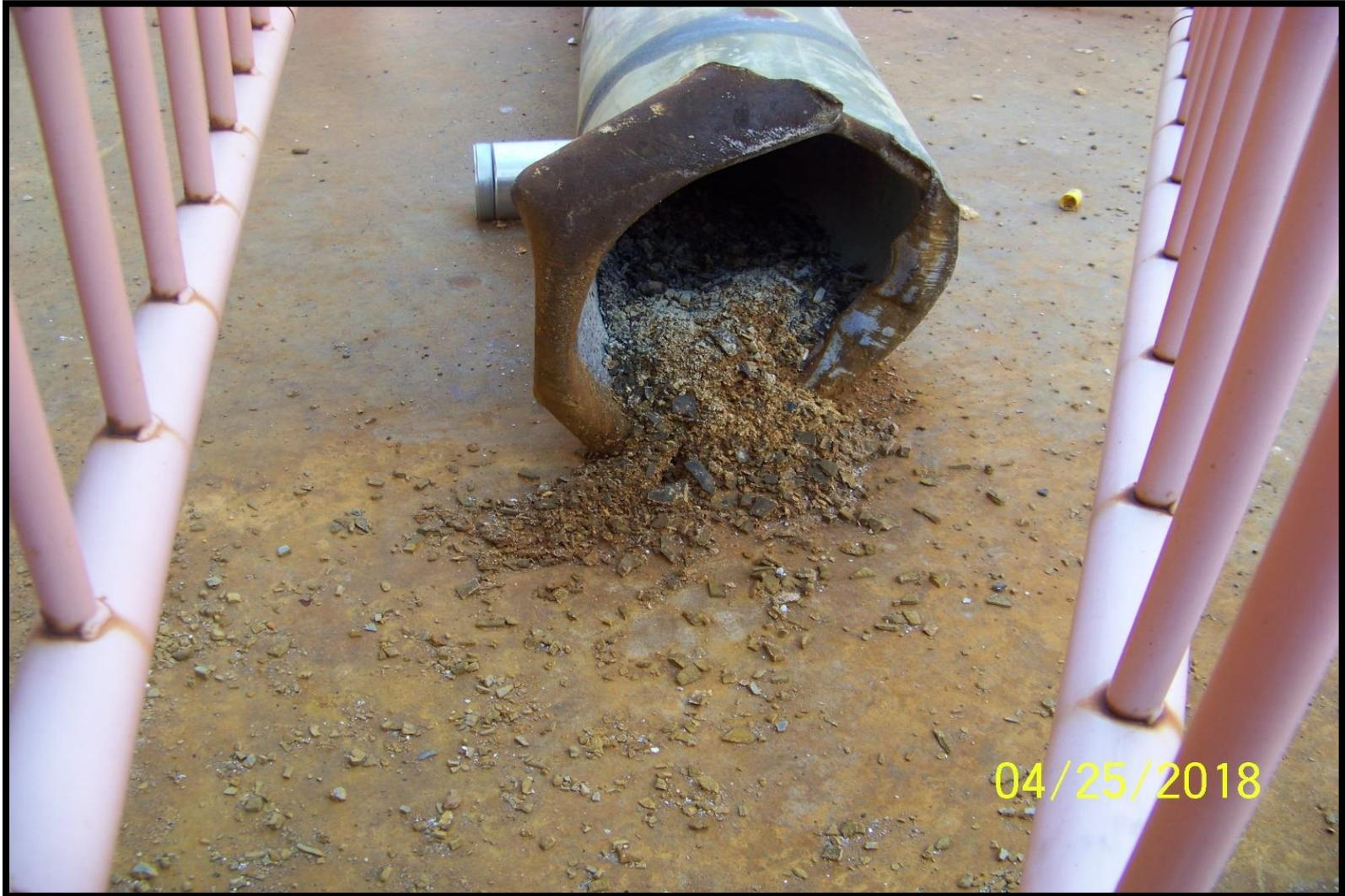
Photo of thinning walls of the 10" feed piping that fed the Fractionator Tower
