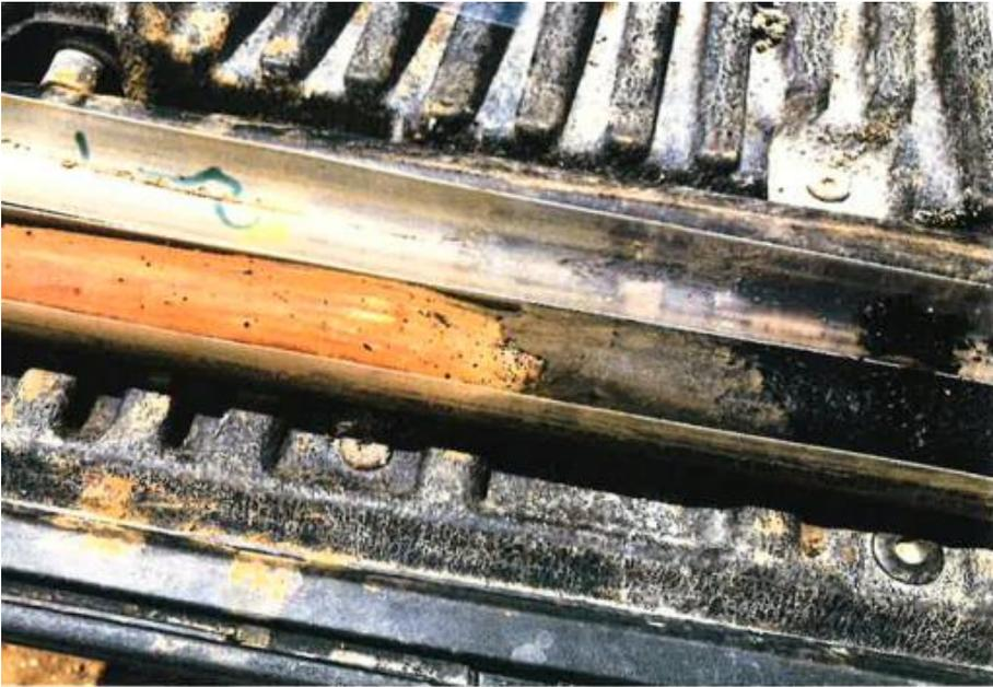
Core from SB-21. Shallower, heavily impacted material on right.
