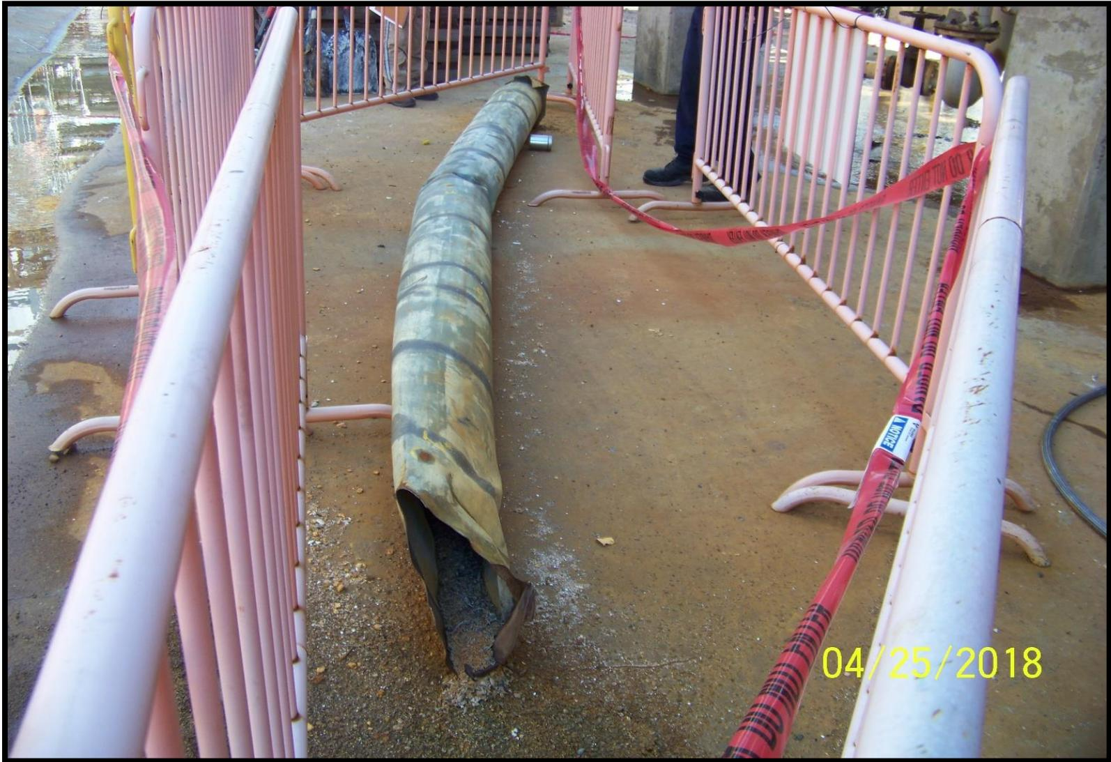
Photo of 16 foot long 10" feed piping that failed and ruptured
