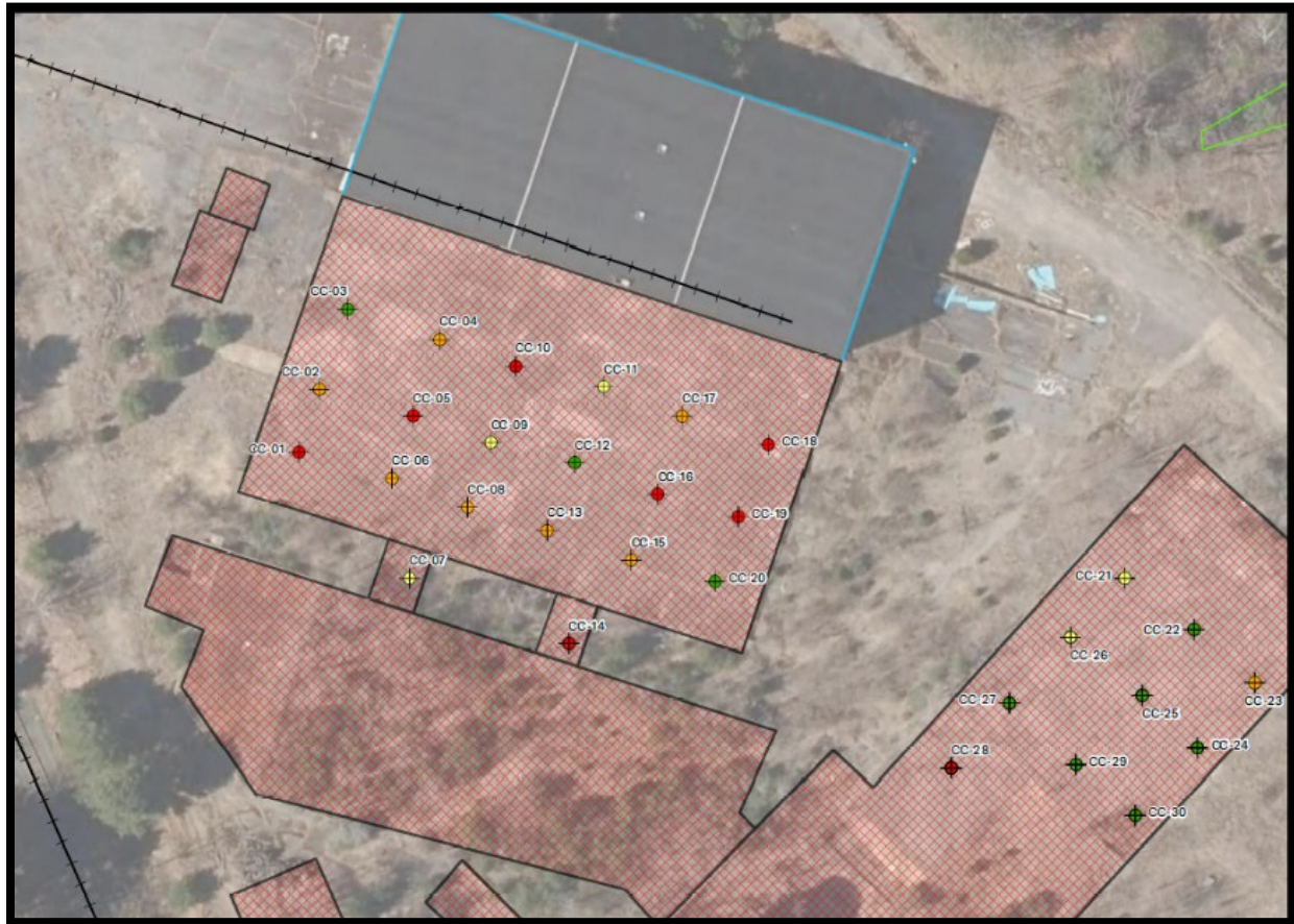
Figure produced as part of Brownfields assessment with concrete sampling locations containing PCBs in excess of 10ppm shown in red.
