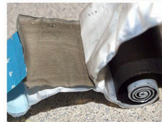
Inside a lithium metal cell
