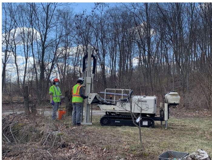
Fig. 1: EPA staff using a Geoprobe to collect soil samples.
