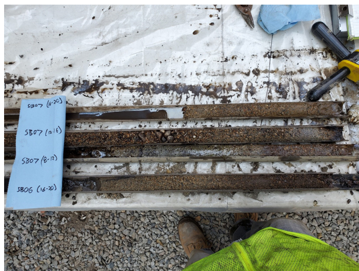
Fig. 2: 4-foot long soil cores.
