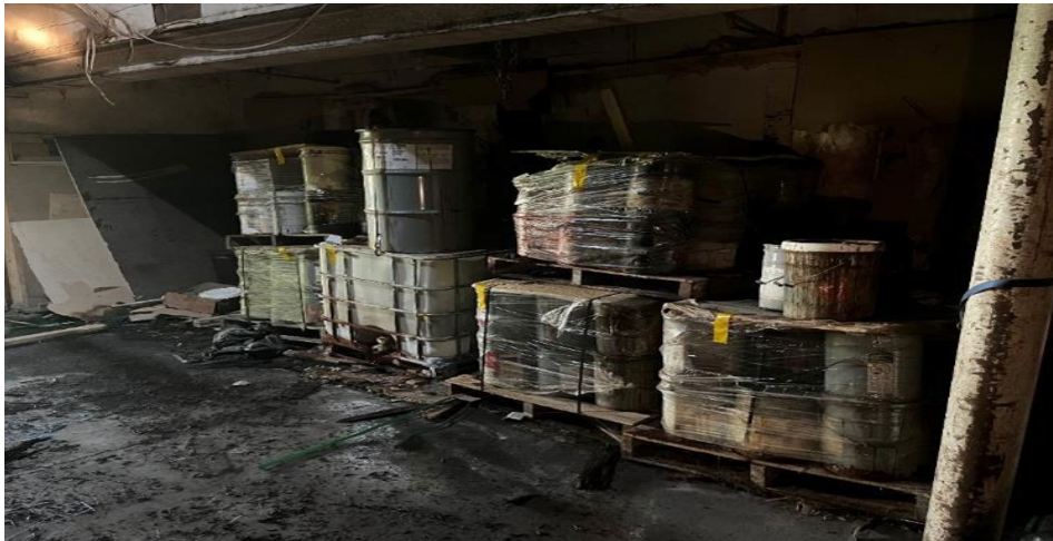
Figure 3: All the drums and containers are visibly corroding or leaking, and many are labeled as flammable.
