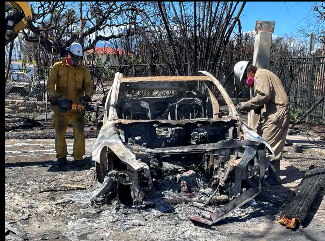
Step 1: Cut Roof/Access Points
