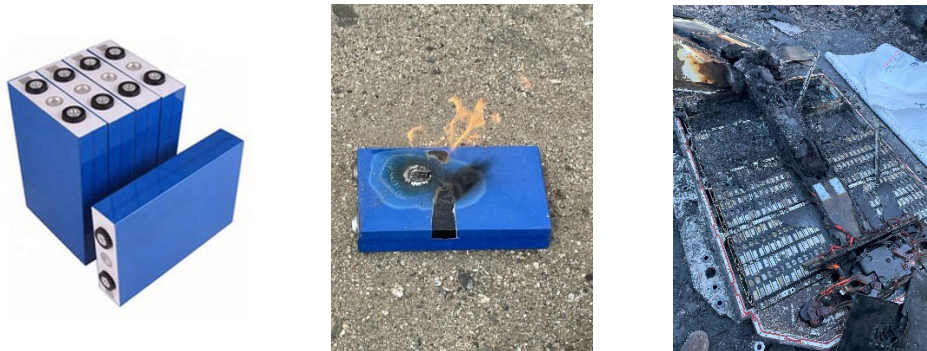
Figure 6. A typical example of a prismatic LIB cell (left), a prismatic cell on fire (center) and a damaged prismatic cell structure EV battery from the 2025 Southern California Wildfire response.
