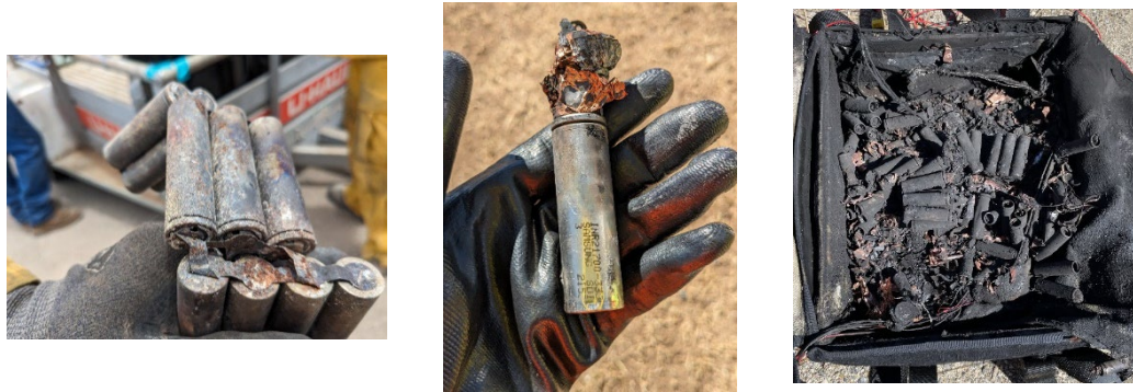
Figure 5. Examples of damaged cylindrical LIB cells
