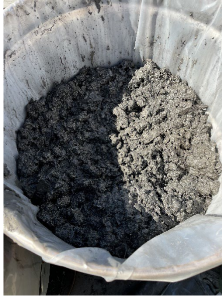
Figure 16. Final product from battery shredder/grinder.
