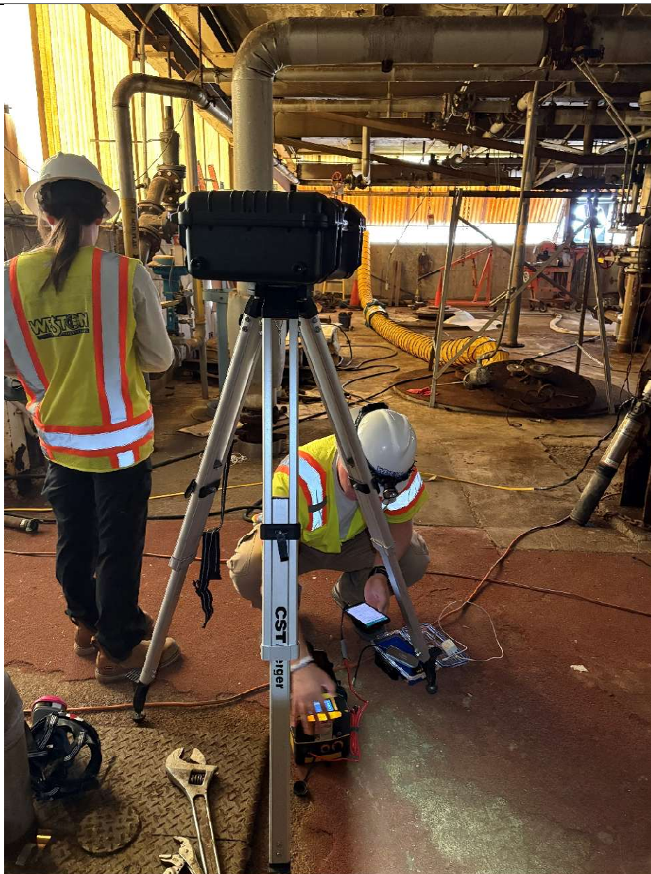
EPA contractors setting up an air monitoring station to assess the interior atmosphere during building venting operations.
