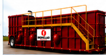
18,000 GALLON FRAC TANK Receives treated liquor from treatment trailer 3" SUBMERSIBLE PUMP - feeds Second Frac Tank CENTRIFUGAL PUMP (rear low port) - plumbed to 20 yard roll-off bin for sludge control
