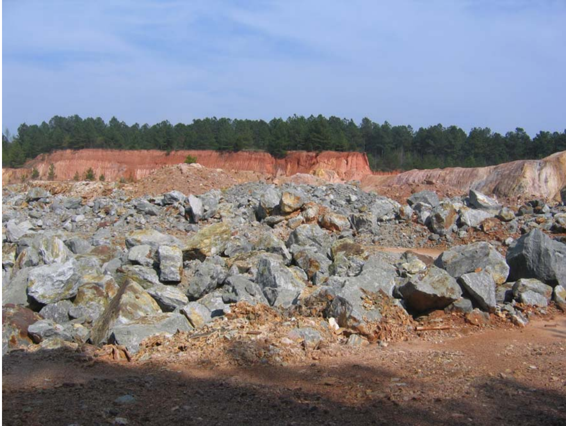
Figure 15. Close-up view of some of the pyrite-containing waste rock piles dumped onto the upper benches on the west side of the Barite Hill Pit.
