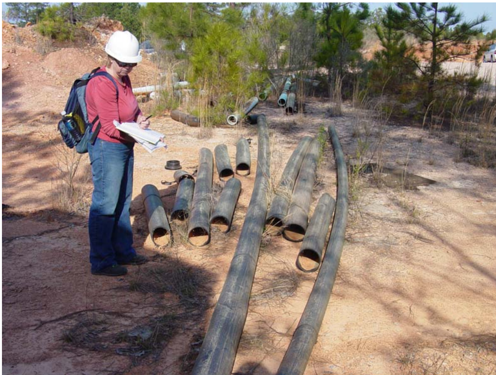
Figure 70. Piles of pipe located near the Mine Office. The HDPE pipe in the foreground should be retained. Pipe in the background is of no value.
