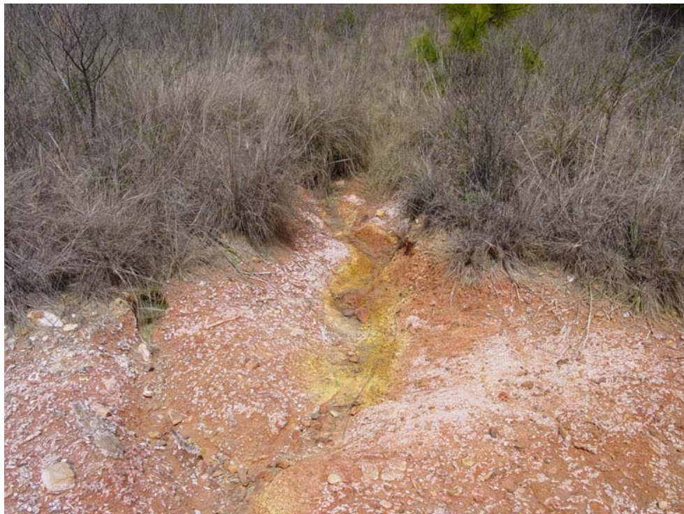
Figure 29. Photograph of the largest of the acid seeps emerging from the southeast side of the Permanent Heap Leach Pad. Yellow staining is the result of precipitation of iron hydroxides. The white coatings on the adjacent bare soil are thought to be the iron sulfate mineral melanterite.
