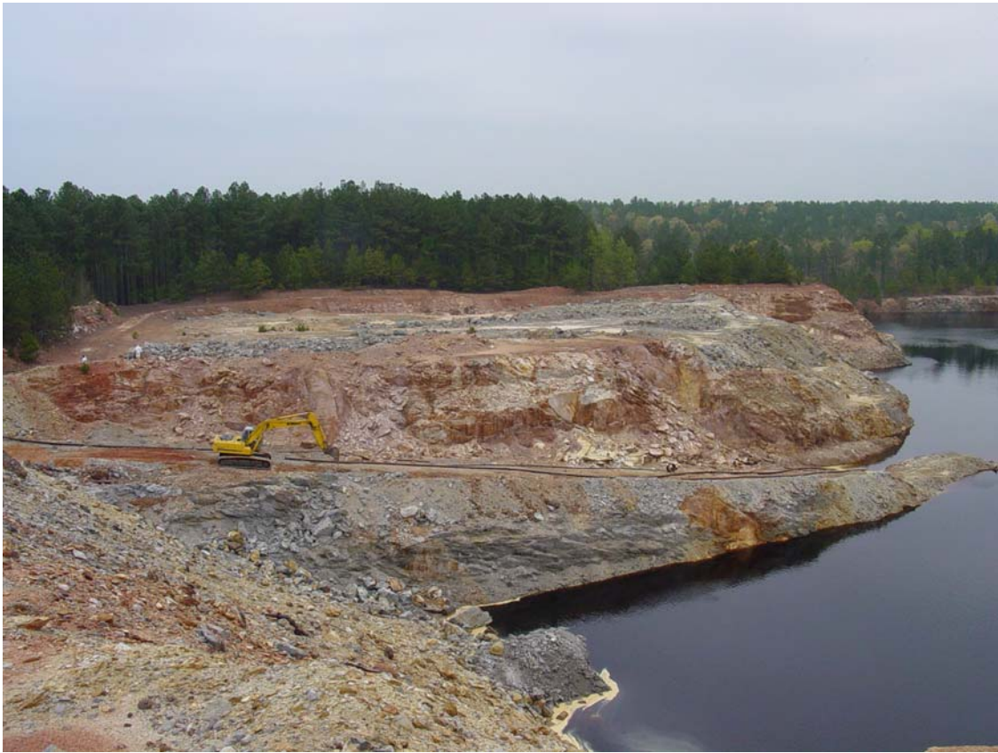
Figure 13. View of grey-colored rocks rich in pyrite on the west side of the pit.
