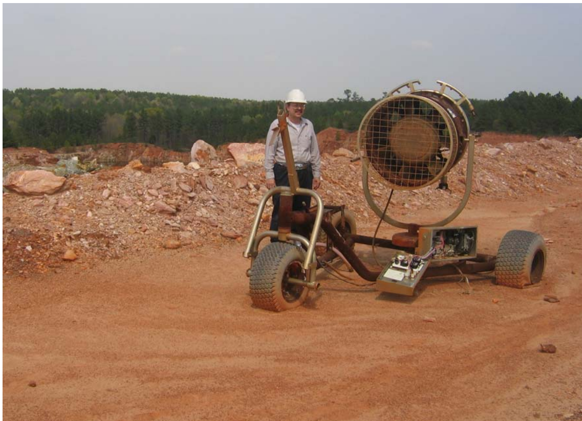
Figure 11. Snow making machine on top of the south highwall was used to evaporate excess site water.
