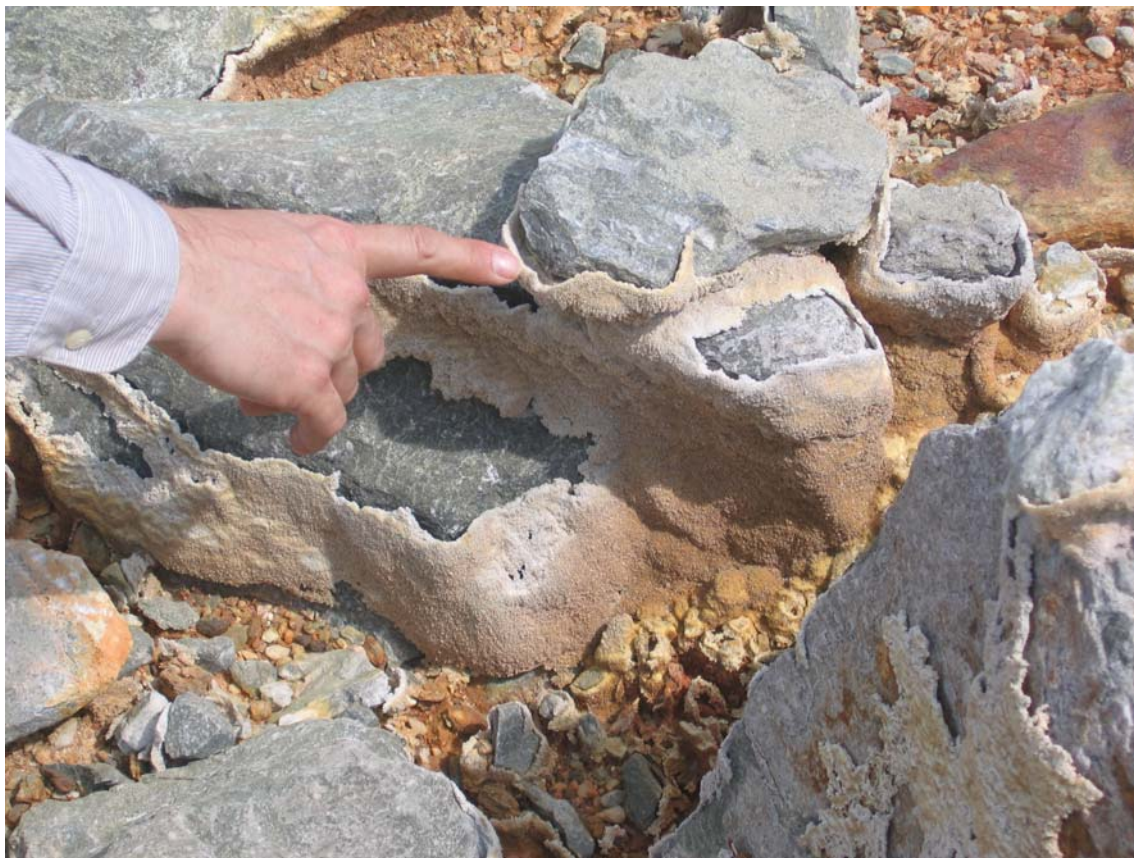
Figure 16. Photograph of damaged “guniting” coating on pyrite-rich waste rock left exposed in the upper benches of the Barite Hill Pit. The coating is a failed attempt to mitigate the acid drainage originating from this waste rock.
