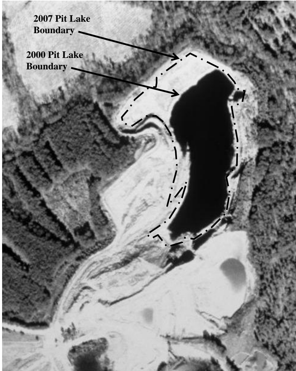
Figure 17. Aerial photograph of the Barite Hill Pit in the year 2000 showing the pit lake about 6 years after mining ended. The pit lake boundary in 2007 (about 12 years after mining ended) has been drawn onto the image.
