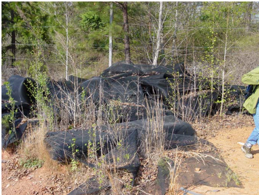
Figure 68. Discarded geonet drain material lies next to the Contingency Pond.
