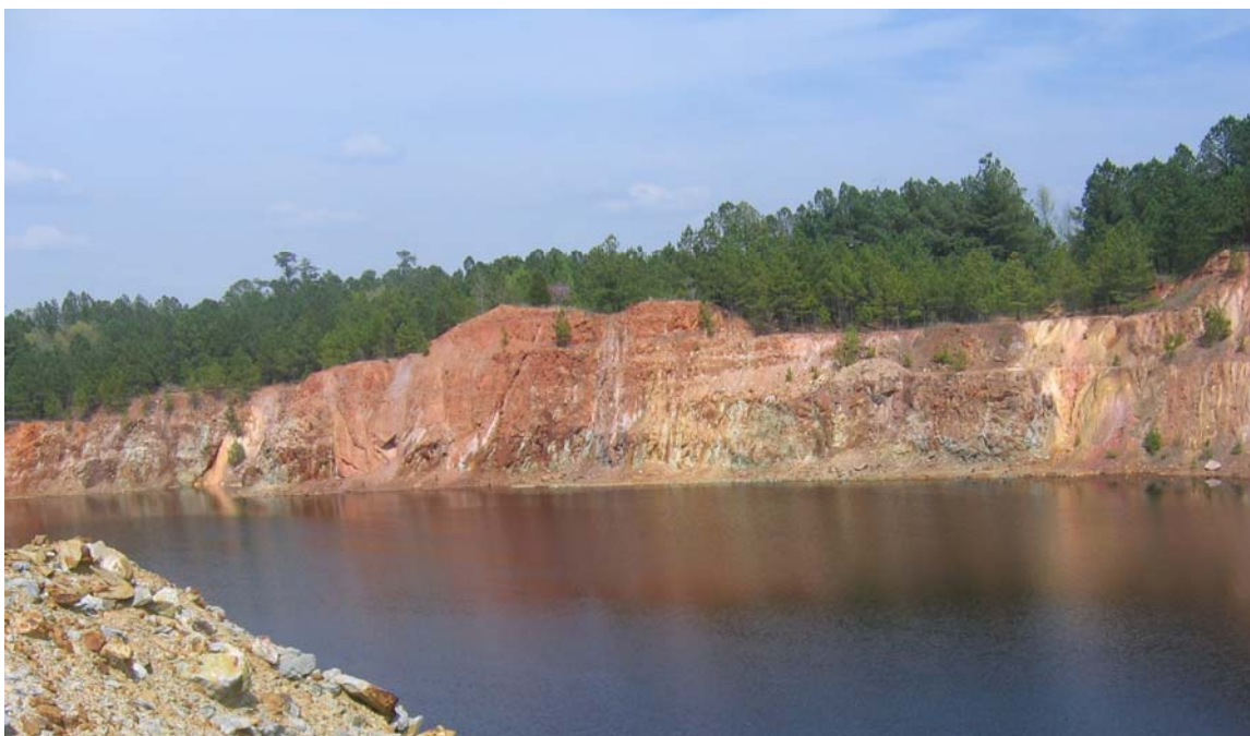
Figure 12. Photograph of the highwall on the northeast side of the pit. The grey to yellow rocks in the highwall are acid generating rock. The red colored rocks and overlying soil likely do not generate acid and show volunteer vegetation.
