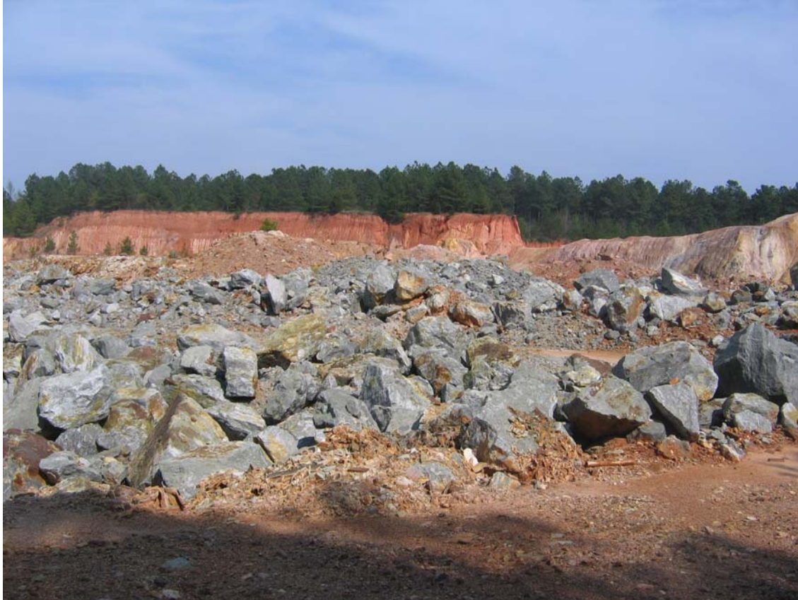
Figure 6. Close-up view of some of the pyrite-containing waste rock piles dumped onto the upper benches on the west side of the Barite Hill Pit.
