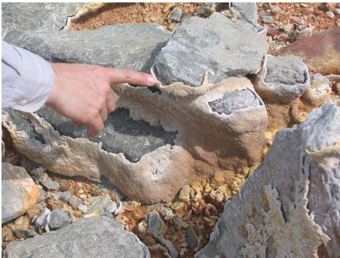
Figure 7. Photograph of damaged “gunite” coating on pyrite-rich waste rock left exposed in the upper benches of the Barite Hill Pit. The coating is a failed attempt to mitigate the acid drainage originating from this waste rock.
