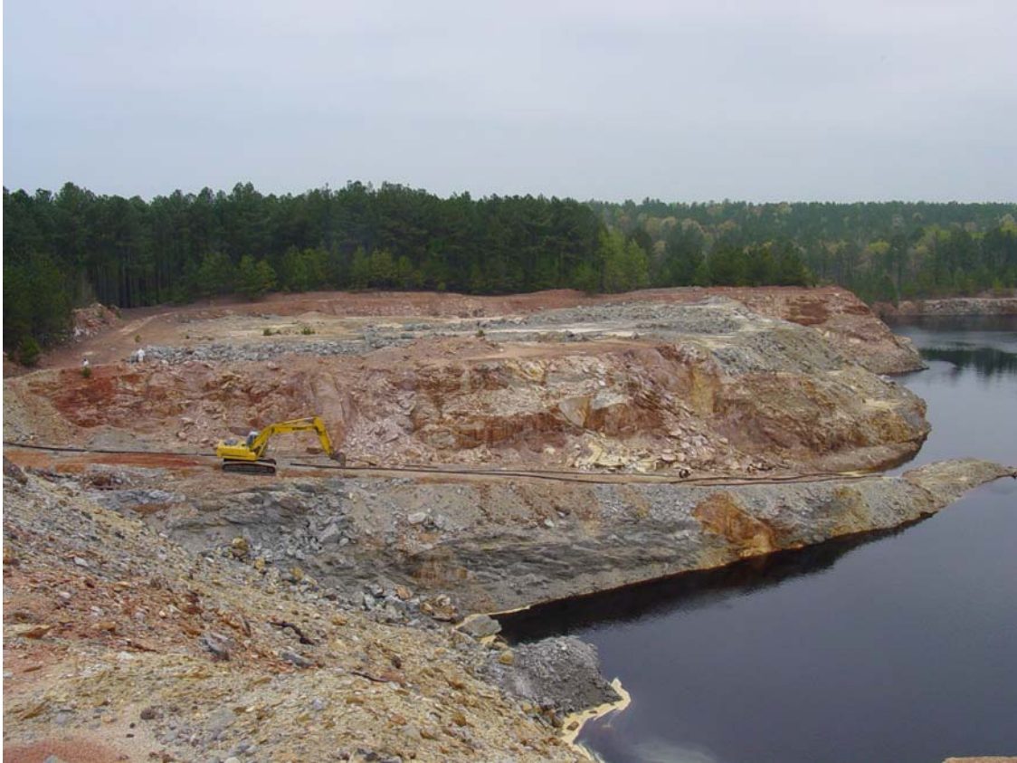
Figure 4. View of grey-colored rocks rich in pyrite on the west side of the pit. The south backfill is seen in the lower left part of the photograph.
