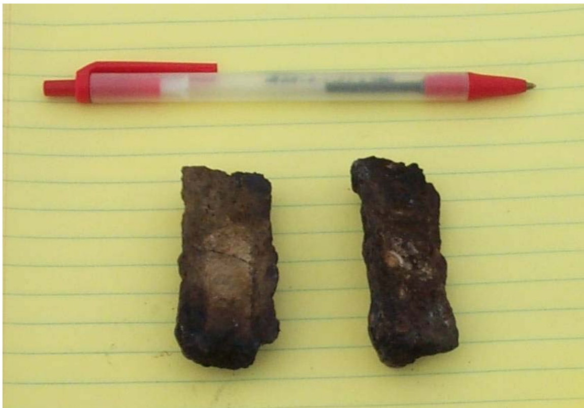
Figure 4 Split 2-inch Tracer Element
