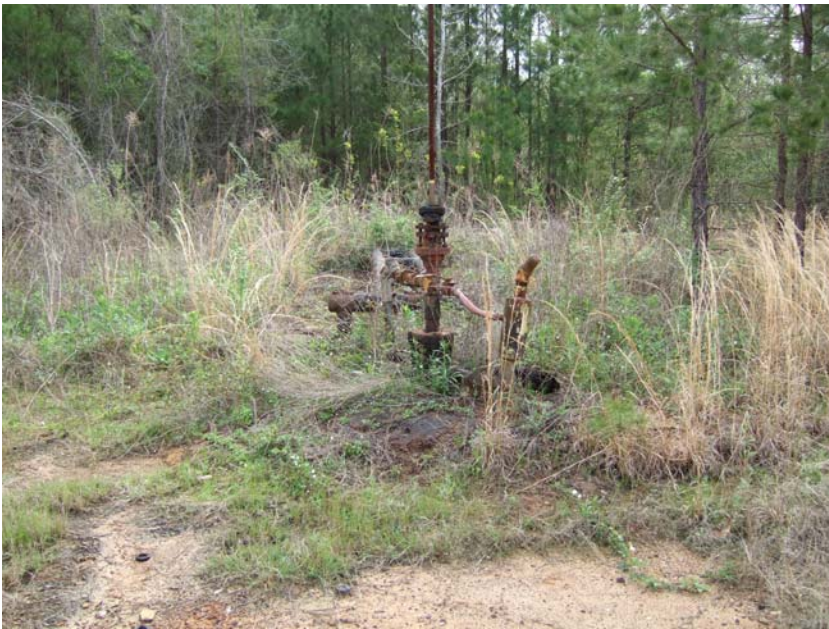
Site Name: Quality Petroleum, Inc.-Hoffman, et al. Project No.: E06614 Photo No.: 0217 Direction: E Contract No. Date: 04/05/2008 Time: 9:48:00 AM Photographer/Witness: Sekerka, Robert/Johnson, Colin Description: E06614: Pump jack stand for Hoffman, et al. Well No. 001 (SN 179621).
