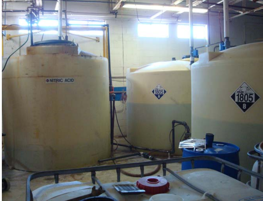
Photograph No.: 3 Photographer: Greg Haas TDD Number: S05-0810-004 Site Name & Location: Lab Tech Industries, Detroit, Wayne County, Michigan Date: October 30, 2008 Subject: Acid Storage in Fiber AST's.
