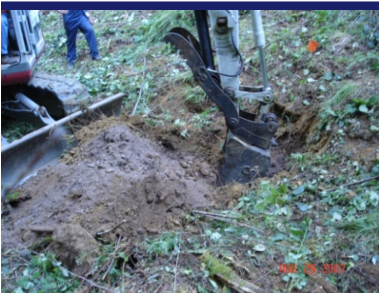
Photo 60 Furnace Creek test hole to determine depth of contamination. Showing ash layer high in mercury.
