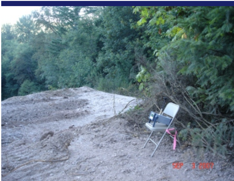
Photo 10 Dataram monitoring air at top of Main Tailings Pile - West slope.
