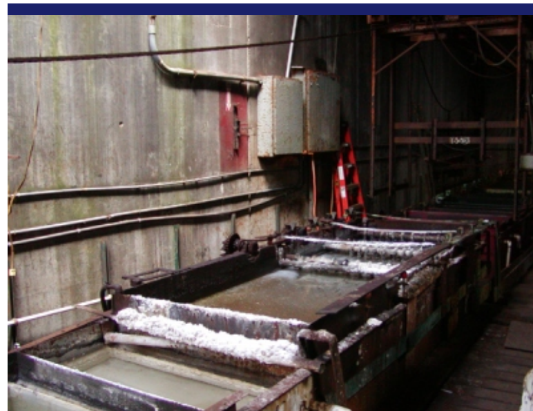
Photo 6 MPA: Plating Line No. 1 (along west wall of main plating area) and power box.
