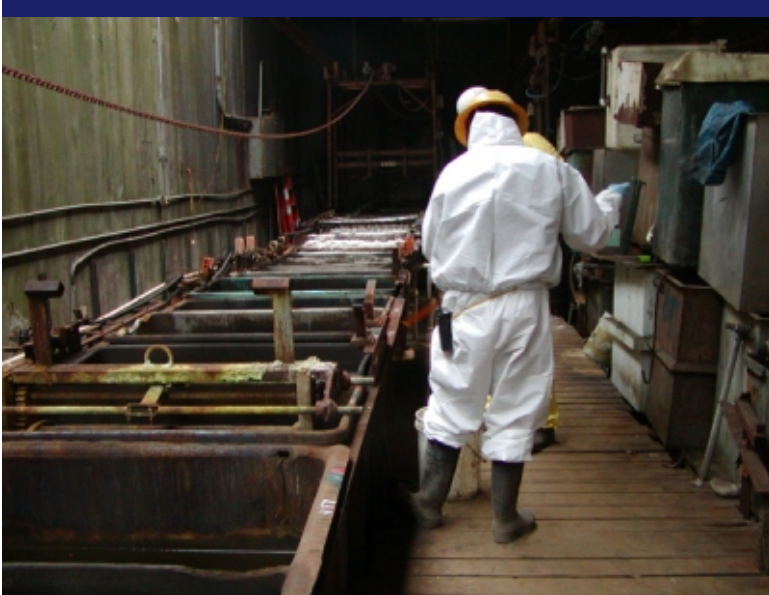
Photo 45 MPA: ERRS conducting compatibility tests on vats.
