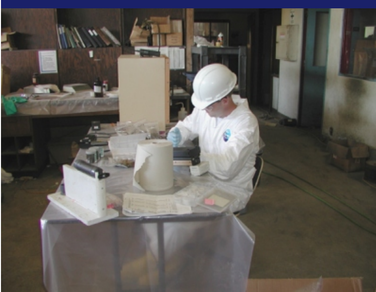
Photo 57 OA: START-2 preparing soil samples for XRF field screening.
