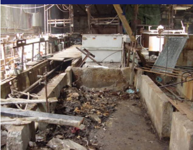
Photo 53 MPA: Sludge and debris beneath plating line 2, main plating area.
