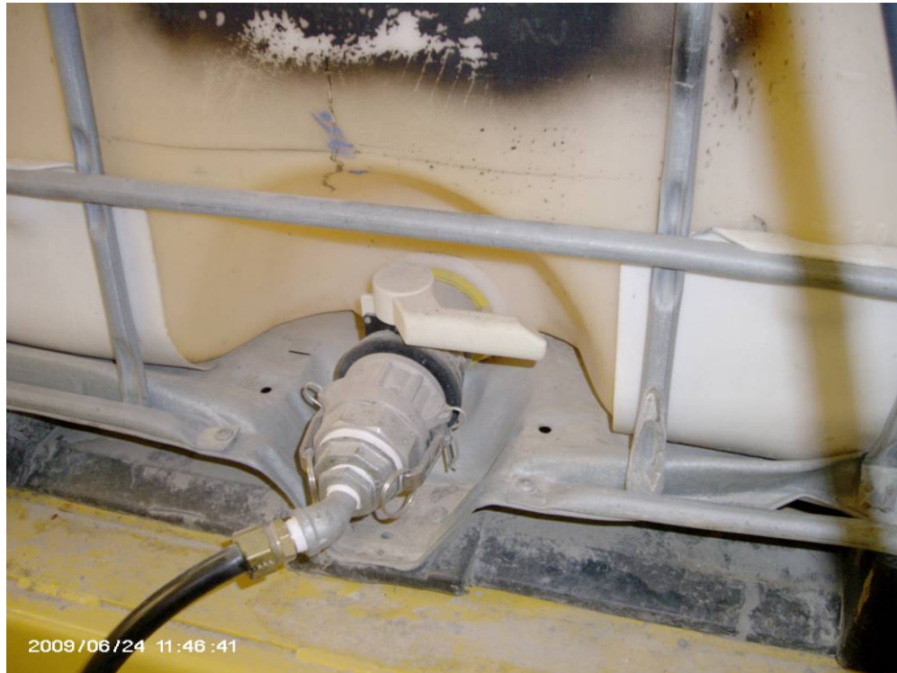
Defoamer Picture 3 – Feed hose cam lok connection and tote outlet valve.
