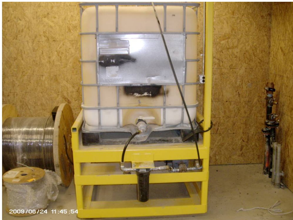
Defoamer Picture 2 – 275 gallon tote tank mixing vessel. Water supply valve is shown in corner on right side of picture.
