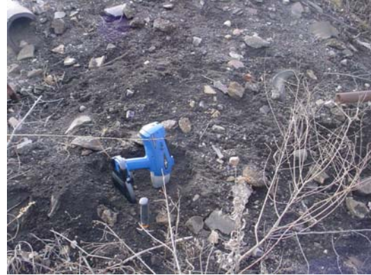
An XRF analyzer used for field screening.
