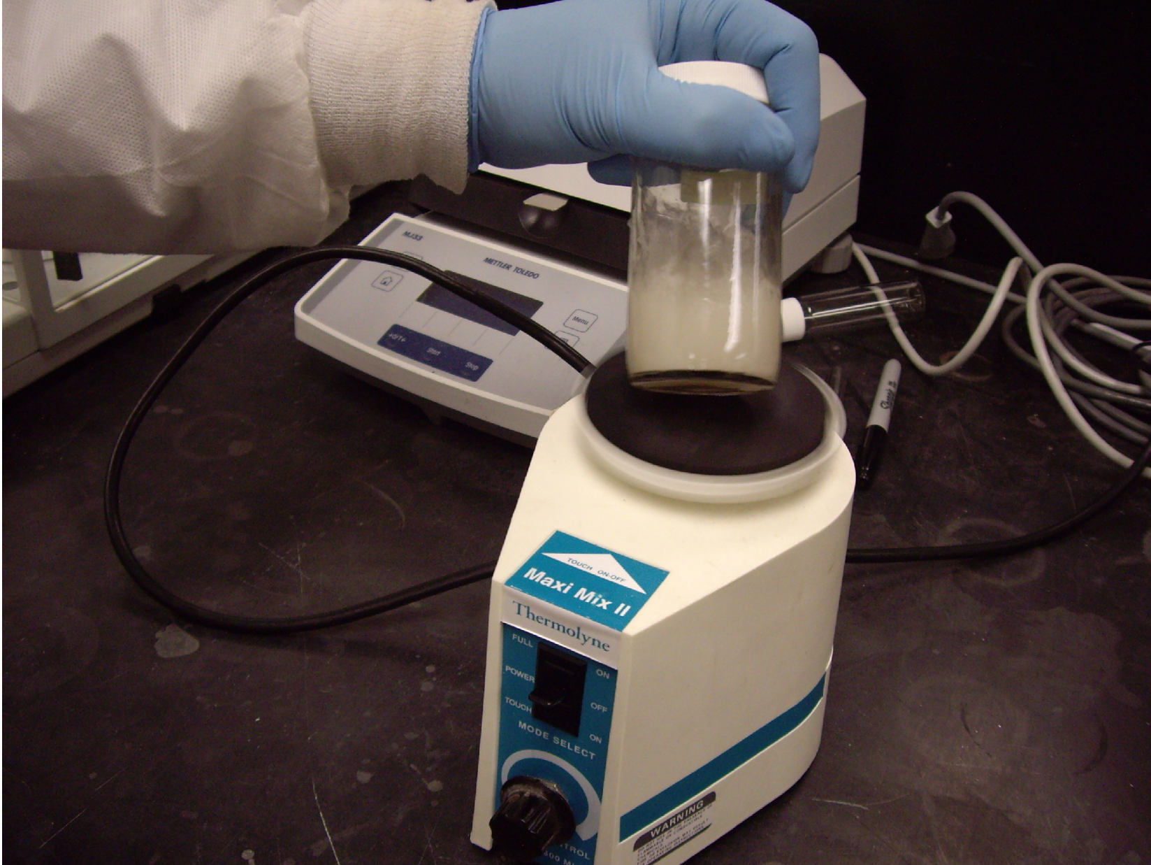
Vortex Extraction - 1 gm drywall in 5ml hexane
