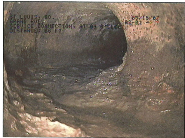
IMAGE: 39a, TAPE #: EMA-1, 00:47:54 66FT, service connection, at 09 o'clock
