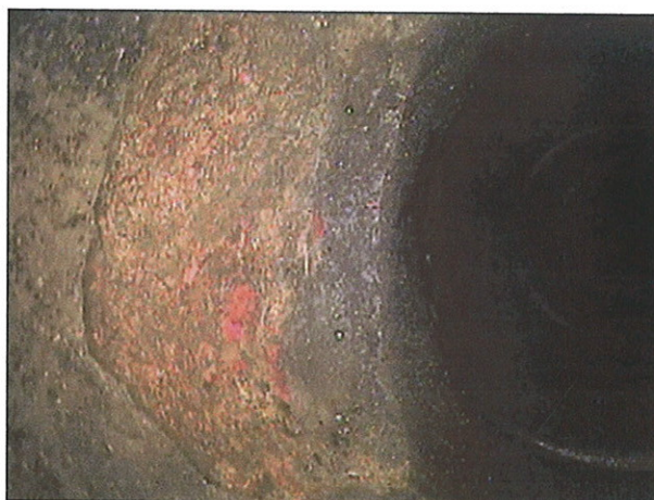
IMAGE: 79b, TAPE #: EMA-1, 01:14:34 286.4FT, Hole in pipe from 11 to 01 o'clock, REMARK: PATCHED
