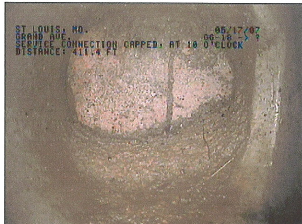
IMAGE: 94a, TAPE #: EMA-1, 01:22:11 411.4FT, service connection capped, at 10 o'clock
