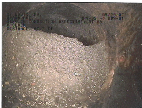
IMAGE: 184a, TAPE #: EMA-1, 02:25:30 67.7FT, service connection defective, at 09 o'clock
