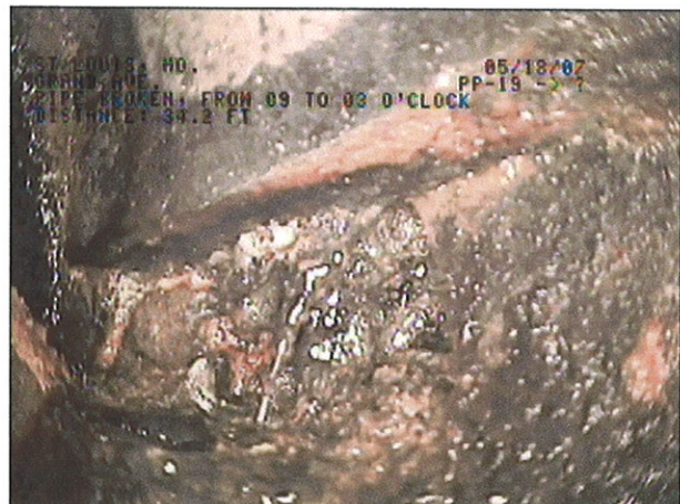
IMAGE: 118a, TAPE #: EMA-1, 01:40:53 34.2FT, pipe Broken, from 09 to 03 o'clock
