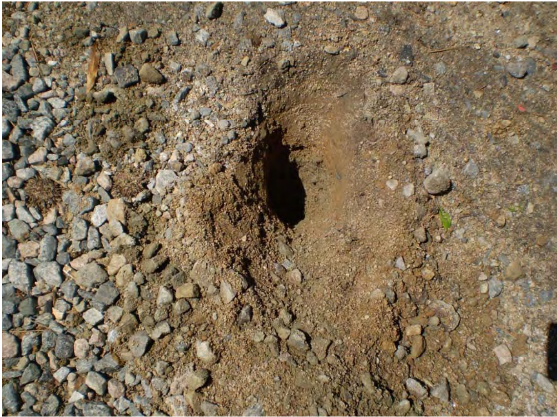
Photograph 3. Boring for one of the four locations used to prepare composite PSALMS ST. B. Shows approximate depth of gravel/battery chips.
