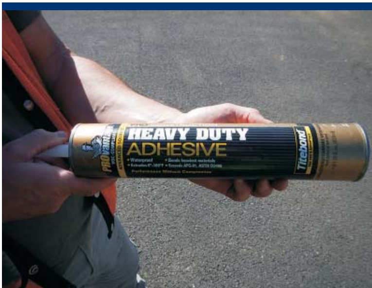
Photo 79 Adhesive used to set top block along retaining wall and parking space stoppers.
