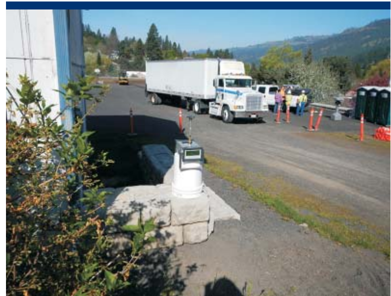
Photo 4 DataRAM (#1) dust monitor; materials being delivered in background.
