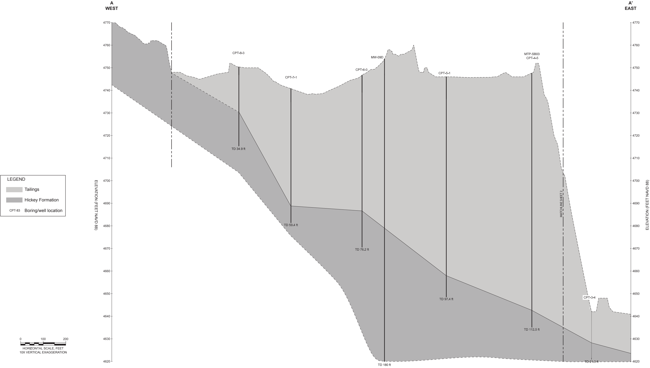
FIGURE 7-12 Iron King Mine Main Tailings Pile Cross Section A-A' (Sheet 1 of 2) Iron King Mine – Humboldt Smelter Superfund Site Dewey-Humboldt, Yavapai County, Arizona
