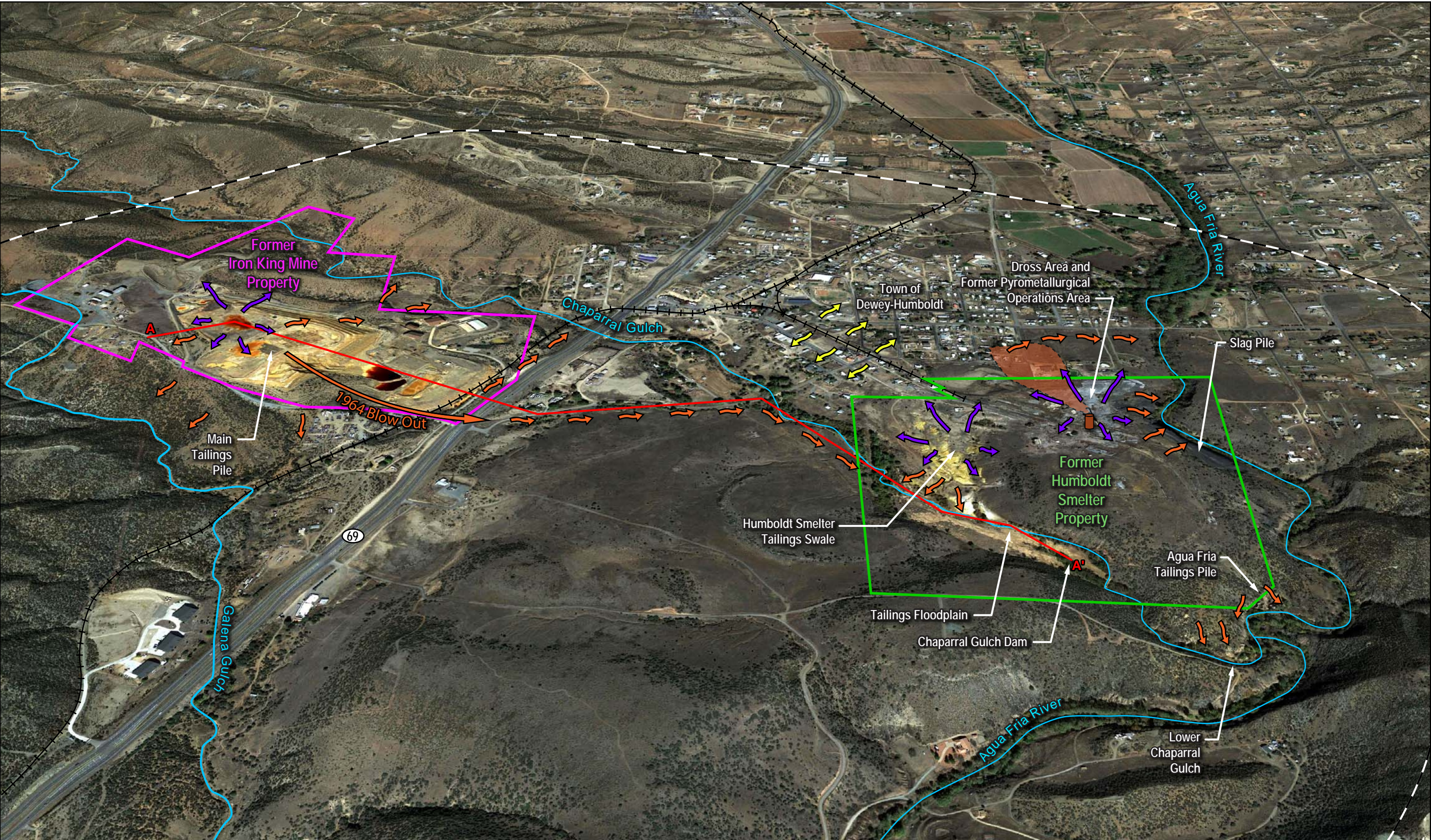
Figure ES-6 Contaminant Transport Mechanisms Iron King Mine – Humboldt Smelter Superfund Site Dewey-Humboldt, Yavapai County, Arizona
