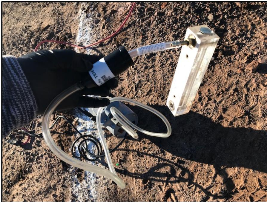
Photo 2: Setting calibration for pump volume
