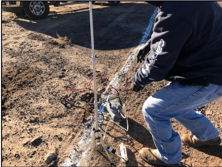
Photo 1: Setting up pumps and cassettes for air samples
