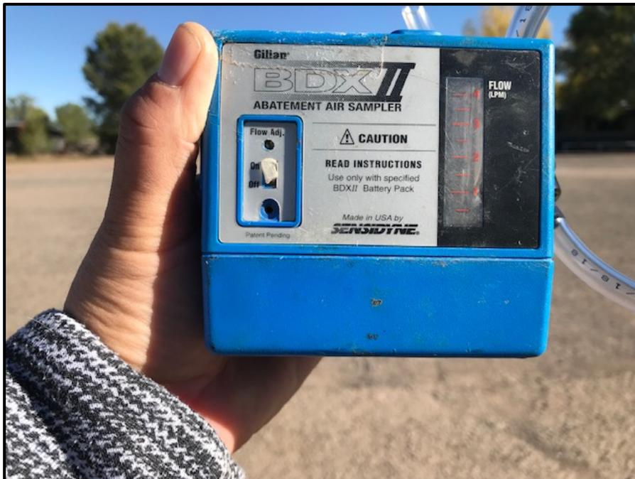
Photo 6: Abatement Air Sampler was used to collect dust samples inside buildings.
