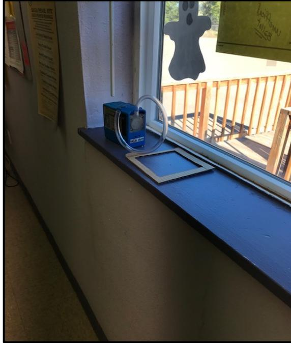
Photo 7: Sampler with a 10 cm X 10 cm guide to aide in collecting 100 cm square area of dust.
