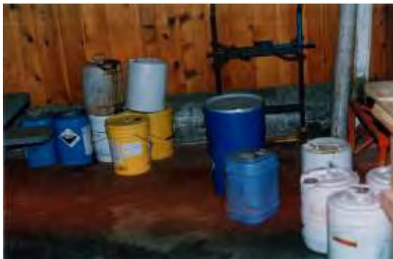
In most of the equipment and maintenance shops, 5-gallon metal or plastic buckets and 55-gallon barrels with unknown contents were observed. These abandoned containers may contain adhesives, solvents, spent oil, and/or gasoline. The containers did not have labels or markings to identify the contents. No staining was evident around these containers although some containers did not have lids.
