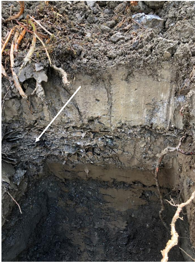
Photograph 3 – Test Pit 1 – Cementitious panel debris (typical) below grade (ACM).
