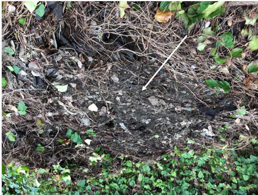
Photograph 4 – East slope – Cementitious panel and vinyl floor tile debris (typical) (ACM).
