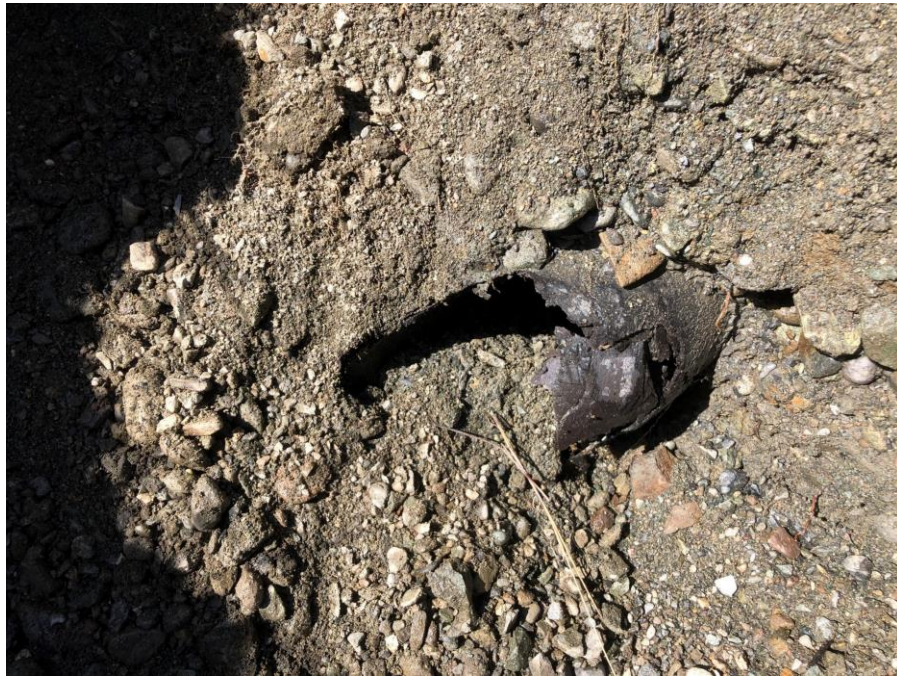
Photograph 5 – Test Pit 10 – Bituminous piping reported to be nondetect (not asbestos).
