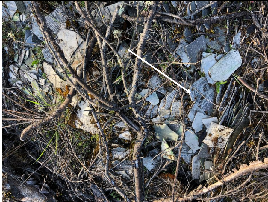
Photograph 1 – Northeast debris pile – Cementitious panel debris reported to contain asbestos.
