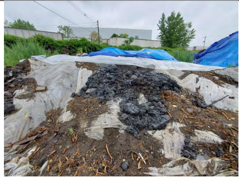
Photo 2: Soil Pile S1 center location with PID reading and Petroleum Staining
