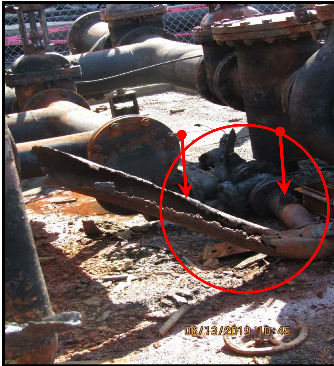
Photo of the partial 2 inch butane injection piping at the manifold - noting rupture at feed piping
